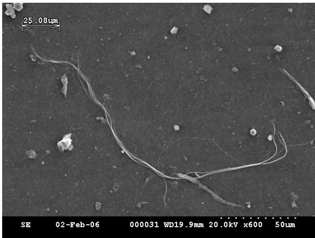
Figure 2.2 Scanning electron micrograph showing chrysotile asbestos fibres
