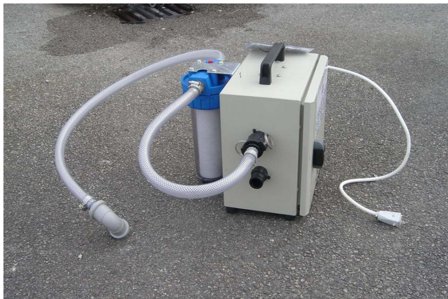
Figure 8.1 Water filtration for the discharge from the decontamination unit. Photograph provided by the UK HSE.
